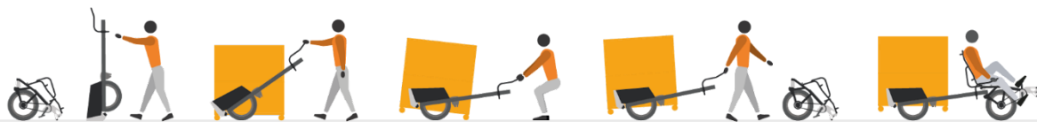
Figure 18: visual explaining the adaptation of the Lift system on the Tricy, source: FLEX
